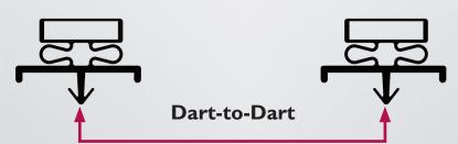
A simple way to be sure of getting an accurate measurement is to measure from the center of the grooves, or from the outside of one side to the inside of the other (see below).
